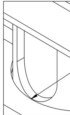
Match radii of cable access hole with ② top and bottom and weld in place
