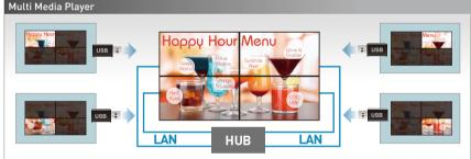
Connecting more than one unit with LAN cable reproduces files in USB memory simultaneously. One of the units becomes Master, and the others Slaves \*For Media Player, provide the following files in USB memory. Play file / Scenario / File list
