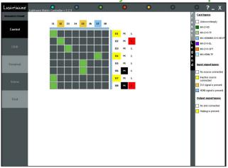
Controls all functions of the router like IP configuration, routing, EDID Management, system status monitoring, Color space and color range control, audio samle rate conversion, etc.
