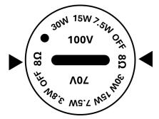
• To set the speaker to a high impedance mode set the transformer tap to the desired power rating as shown in the picture. In this example, if the speaker will be connected to a 100V line its power rating will be 30W and if connected to a 70V line its power rating will 15W.
