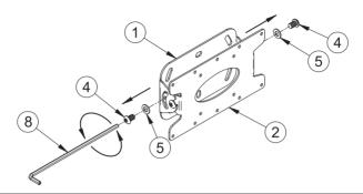
ii. Loosen the front set of M8 x 12mm (part 4) screws and lift off interface plate (part 2).
