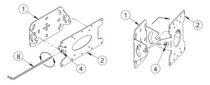
iii. Position the front set of M8 x 12mm screws (part 4) on interface plate (part 2) as shown.
