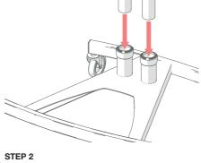
Place base upside down on the floor. Locate castors and push into the four holes until they click into place.
