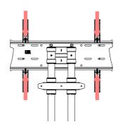
Using another team member, lift the screen up and gradually offer it up to the back plate. Gently tilting the screen forward, hook the arms over the rail of the back plate and lower into position.
