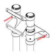
Decide where the product is to be installed. Measure 102.5mm out from wall (not skirting) mark, drill and secure the floor plate into position. (Fixings not supplied).
