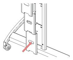
Identify remaining mast in-fill panels. Start from the bottom and clip 2 of the 3 larger rear panels in, threading cabling through where necessary.
