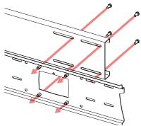
Once placed over columns and at the desired height, tighten the two grub screws to secure into place. Tighten up the base grub screws to secure.
