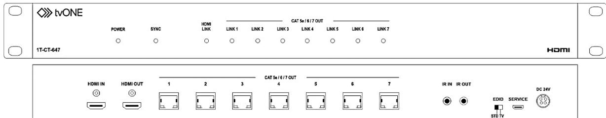
1. Connect the HDMI source device's output to the HDMI IN connector of the 1T-CT-647 Transmitter, using an appropriate HDMI cable, (10 Meter (~30') in length for 12 bit signals, 15 meters (~45') for 8 bit signals).
