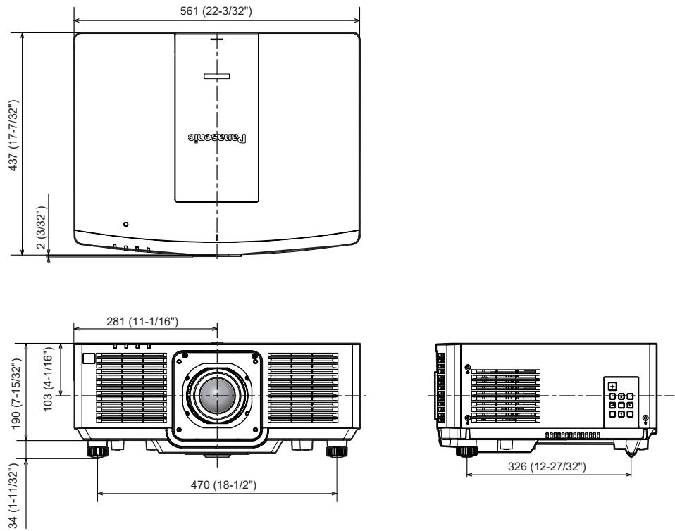
\* The above dimensions are obtained when the standard zoom lens or the optional zoom lens (Model No.: ET-ELS20) is attached.
