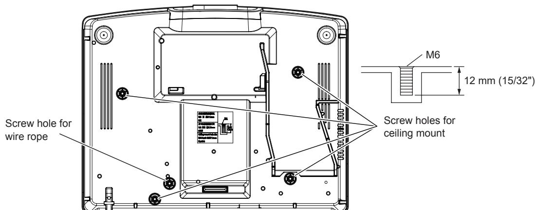
■ Dimensions for the screw holes to fix the projector (projector bottom view)
