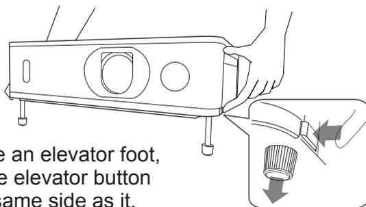
To loose an elevator foot, push the elevator button on the same side as it.
