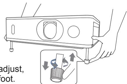
To finely adjust, twist the foot.
