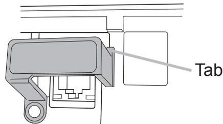
3. Align the screw holes on the projector and the cover. Then insert the screw removed from the projector into the hole and tighten the screw.
