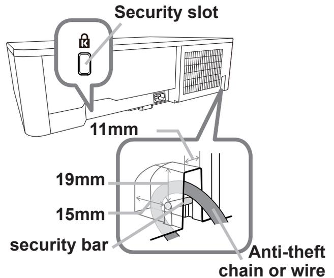
**⚠ WARNING** ► Do not use the security slot to prevent the projector from falling down, since it is not designed for it.
