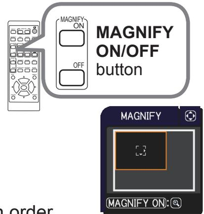
**NOTE** • The MAGNIFY dialog will automatically disappear in several seconds with no operation. The dialog will appear again if the **MAGNIFY ON** button is pressed when the dialog has automatically disappeared.
