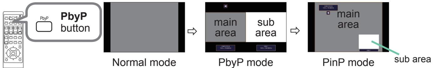
Press the **PbyP** button on the remote control. This activates the PbyP mode. Then, press the **PbyP** button again. The projector goes into PinP mode. The screen displayed before the **PbyP** button was pressed will be displayed as the main area. Most of operations are effective for the main area only. Only outputs the audio input signal paired with the picture input signal for the main area. To quit the PinP mode, press the **PbyP** button again.
