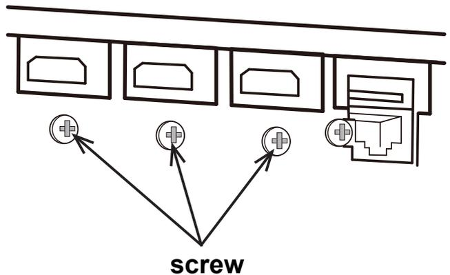
It is recommended to fasten the HDMI cables by using the HDMI cable holder and the Cable tie to prevent them from coming off. Use a Cable tie with the size of 2.0 x 4.0mm or smaller.
