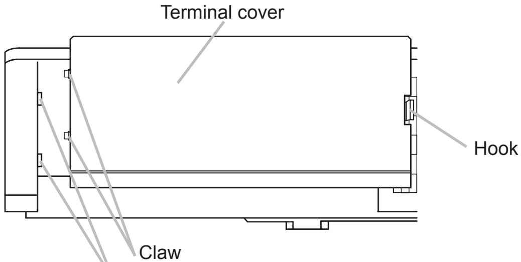
Insert the two claws of the Terminal cover into the hole of the case and confirm Hook is fitting into the case.
