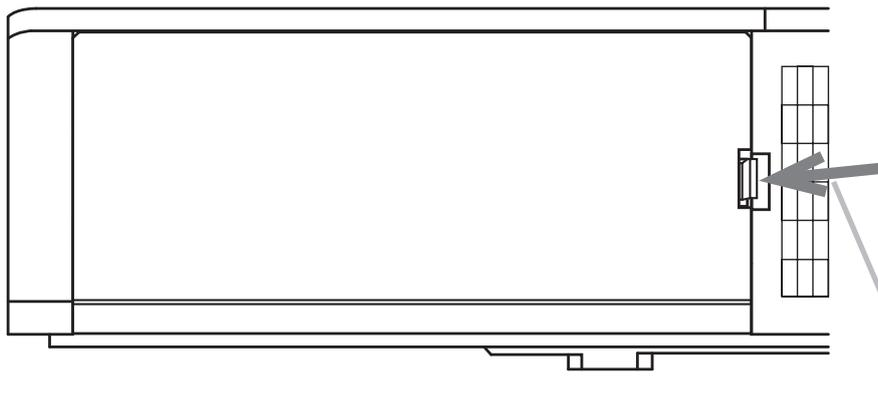
When detaching the Terminal cover, push the Hook in the direction of the arrow and pull it forward.
