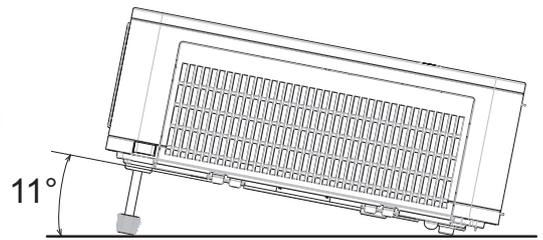
This projector has 2 elevator feet and 2 elevator buttons. An elevator foot is adjustable while pushing the elevator button on the same side as it.
