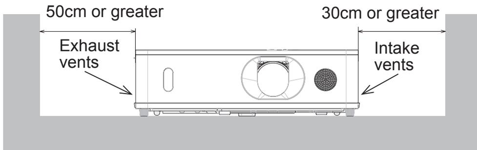
Secure a clearance of 30cm or greater between the intake vents and walls. Assume that there is enough clearance in the front, sides, and top of the projector in the figure below.
