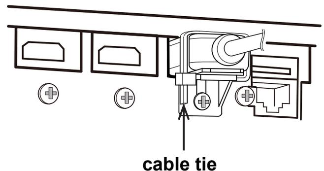
**⚠ WARNING** ▶ Do not fasten the cables other than HDMI.
