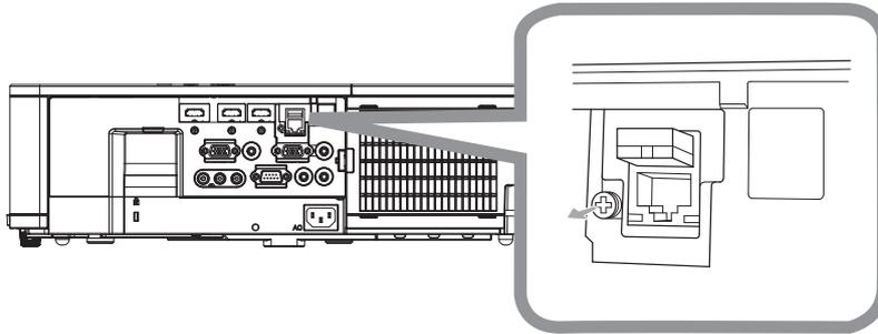
2. Insert the tab of the cover into the hole at the upper right of the **WIRELESS** port in the direction of the arrow.
