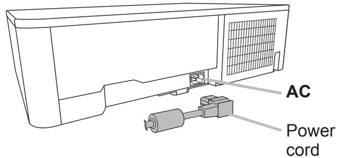
2. Firmly plug the power cord's plug into the outlet. In a couple of seconds after the power supply connection, the **POWER** indicator will light up in steady orange.
