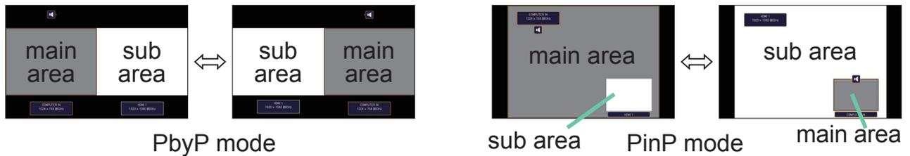
**NOTE** • For some signals, it may not be displayed correctly in the PbyP / PinP mode, even if it can be displayed properly in the normal mode.
