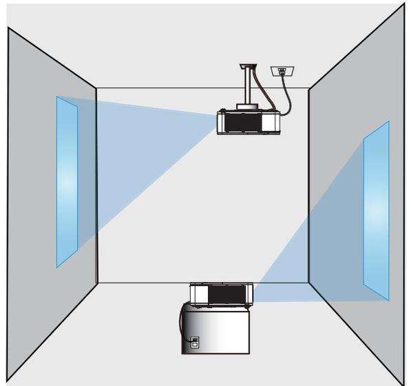
Secure a clearance of 50cm or greater between the exhaust vents and walls, and a clearance of 30cm or greater between the intake vents and walls. Assume that there is enough clearance in the front, back, and top of the projector in the figure below.
