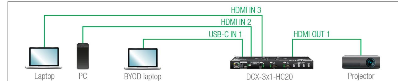
The laptop on HDMI input 3 will be automatically switched to the HDMI output if there is no other source connected to the switcher. If the PC is powered on and has active video signal, the HDMI input 2 will be switched to the HDMI output. If the BYOD Laptop is connected through the USB-C input 1, it will be switched to the HDMI output – independently of the presence of the other video signals.
