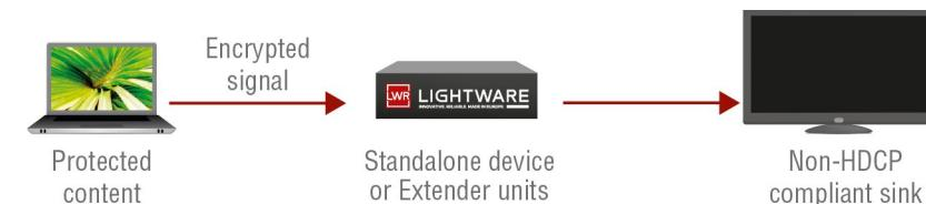
The sink is not HDCP compliant, thus it will not display the video signal, but blank screen is shown. If HDCP is disabled on the input port of the matrix, the source will not send the signal. The solution is to replace the display device with an HDCP-capable one.
