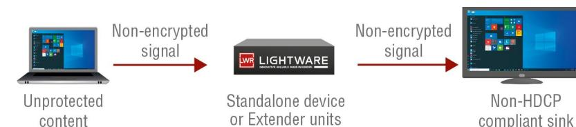
Setting the HDCP parameter to Auto on the output port and disable HDCP on the input port, the transmitted signal will not be encrypted if the content is not protected. Thus, non-HDCP compliant sinks will display non-encrypted signal.
