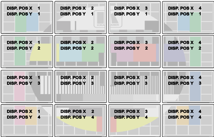
Figure 3: Setting the X and Y Position in a 4x4 Wall Arrangement Matrix
