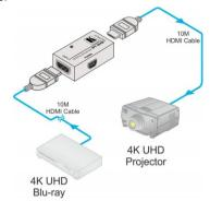
The **PT-3H2** input is connected via a long male-to-male HDMl cable (not provided) to an HDMl source, such as a 4K UHD Blu-ray player.
