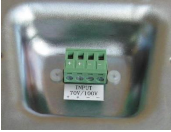
Figure 5: Plugging and Securing the Cable
