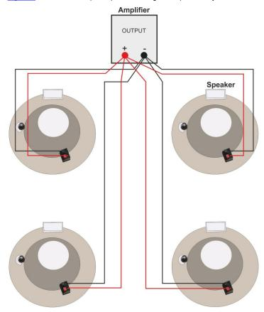
Figure 9 shows an example of parallel wiring in a square array installation:
