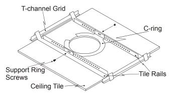
Figure 5: Installing the Open-back Ceiling Speakers
