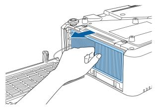
Tap each side of the air filter 4 to 5 times to shake off any excess dust.
