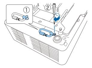
2 Loop the safety wire through the hole in the ceiling mount, and then attach both ends to the carabiner.
