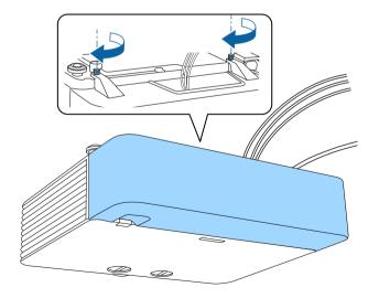
To remove the cover, loosen the cover screws and pull the cover off of the projector.
