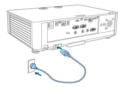
The projector's power indicator turns blue. This indicates that the projector is receiving power, but is not yet turned on (it is in standby mode).
