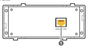
(1) CAT5e/6/7 OUT Port: Connect to a compatible HDBaseT receiver with a single Cat.5e/6/7 cable for transmission of all data signals. Power via PoH will also be supplied to this unit when connected to a compatible PSE receiver.
