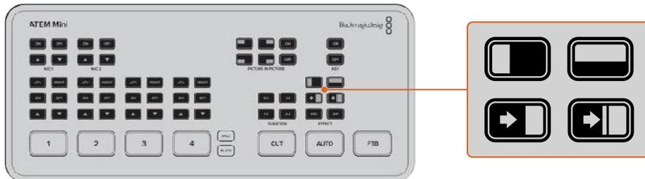
Press the transition type button for the transition you want to use, for example a horizontal or vertical wipe, push or squeeze DVE transition, and mix or dip transition
