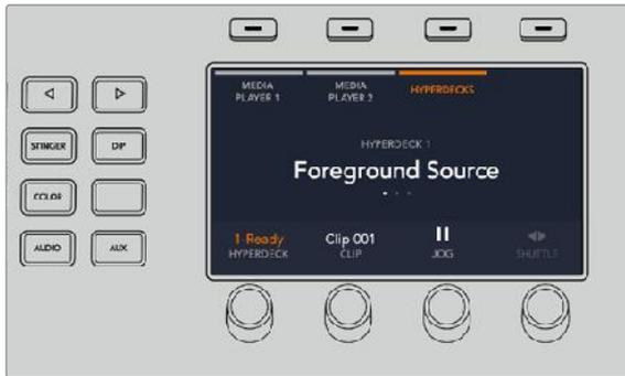
You can now use the rotating knobs below the 'hyperdeck,' 'clip,' 'jog' and 'shuttle' indicators to select HyperDecks, select clips, and jog and shuttle these clips.
