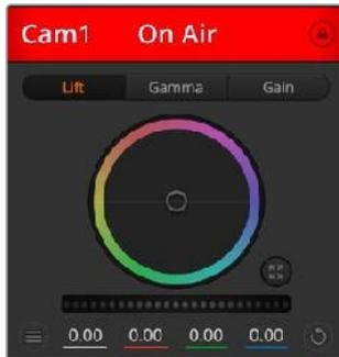
Each camera controller displays the channel status so you know which camera is on air. Use the color wheels to adjust each YRGB channel's lift, gamma and gain settings.
