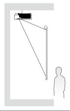
Your room layout or personal preference will dictate which installation location you select. Take into consideration the size and position of your screen, the location of a suitable power outlet, as well as the location and distance between the projector and the rest of your equipment.
