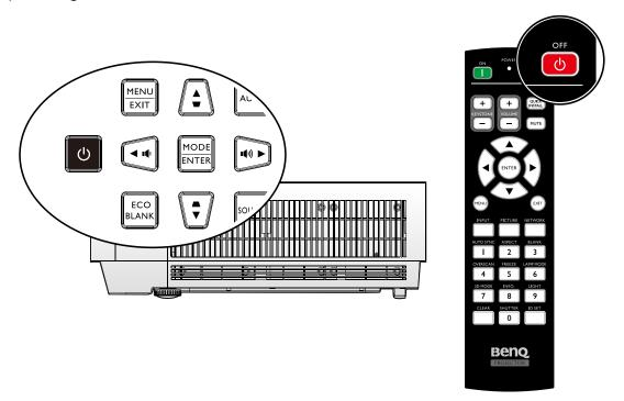
3. Once the cooling process finishes, a "Power Off Ring Tone" will be heard. The POWER indicator light is a steady orange and fans stop. Disconnect the power cord from the power outlet.
