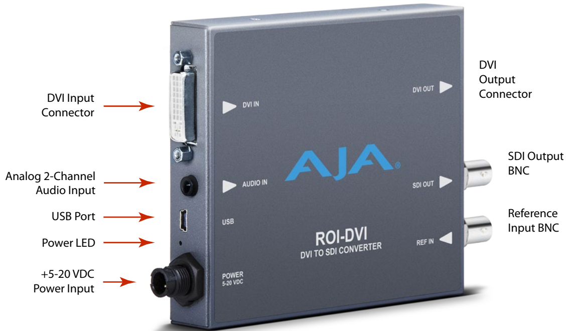
Figure 4. ROI-DVI Converter/Scaler
