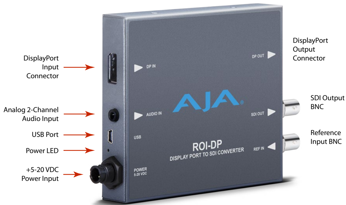
Figure 3. ROI-DP Converter/Scaler
