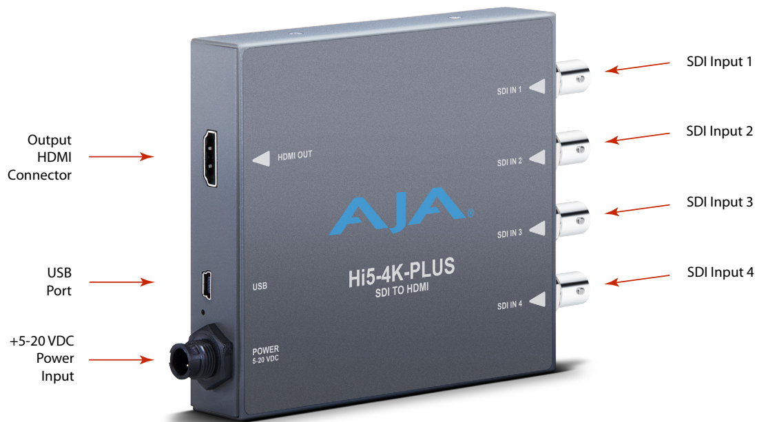
Figure 2. Hi5-4K-Plus Converter Connections
