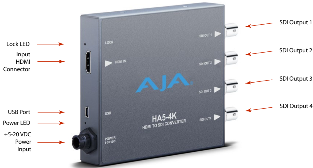
Figure 2. HA5-4K Converter Connections
