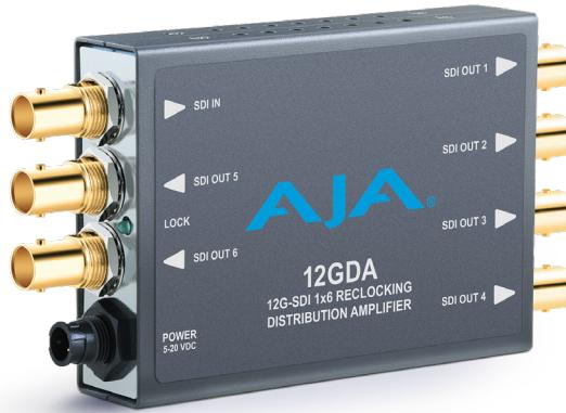
The 12GDA is a miniature, low-cost 1x6 12G-SDI re-clocking distribution amplifier. Featuring six separately buffered SDI outputs, the 12GDA provides automatic cable equalization, re-clocking and input detection.
