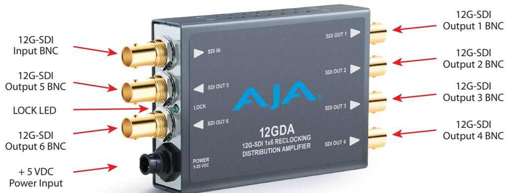
**NOTE:** The LOCK LED indicates valid input video by color: green for SD, red for all other rates, off is no input.
