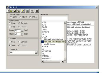
\* There are only 2 x RS232 ports so if you use a lift the closed contact should be used for the screen
