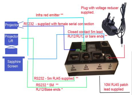
The control panel is powered from the breakout box via the standard 10M Cat 5 cable supplied.
