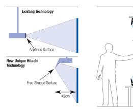
Ultra Short Throw – Using Hitachi's new unique high performance lens. We are able to dramatically reduce the throw distance. combined with the introduction of a high angle projection capability, the quiet ED-A101/ED-A111 projector can be sited only 42cm away for a 60" screen.
