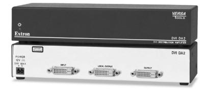
The DVI DA2 is a one input, two output DVI distribution amplifier that allows one single-link DVI signal to be distributed to two displays or other destinations at the same time. The DVI DA2 provides automatic input equalization to ensure optimal image quality on both outputs. It is housed in a 1U, half rack width metal enclosure, and is ideal for use in presentation environments such as classrooms, conference rooms, lecture halls, or wherever reliable DVI signal distribution is needed.
