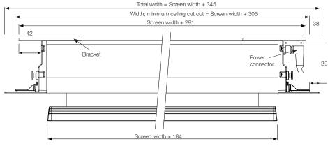
**Considerations regarding cut out width** Minimum cut out width: screen width + 305 Maximum cut out width: screen width + 343
