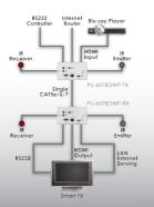
1x HDMI (1x HDMI Uncompressed AV and Data), 1x 9pin Dsub (1x RS-232 Data), 1x 3.5mm Stereo mini-iack (1x Infra Red Receiver
