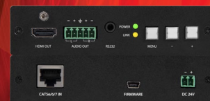
HDBaseT™ Extender/Scaler [model no. AT-HDVS-RX]
