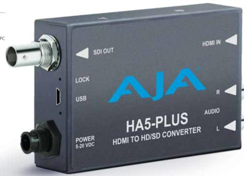
HA5-Plus is AJA's next generation HDMI-to-SDI Mini-Converter. The HDMI input is converted to SD, HD, or 3G-SDI, depending on the input format, for driving SDI equipment. Up to eight channels of HDMI audio are embedded into the SDI output and a 2-channel RCA analog input allows embedding of separate audio into the SDI output, all user configurable. The HA5-Plus also accepts progressive SD (480p, 576p) for compatibility with many DSLR cameras.
