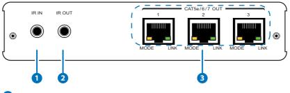
**1 IR IN:** Connect with IR Extender to receive IR signal from Transmitter side and blast out at Receiver side. Ensure that remote controller being used is within the direct line-of-sight of the IR Extender.
